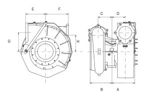
Turbine and compressor washing are catered for. All casings, including suction branches and the gas outlet elbow, are also prepared for the connection of temperature and pressure measurement sensors.
